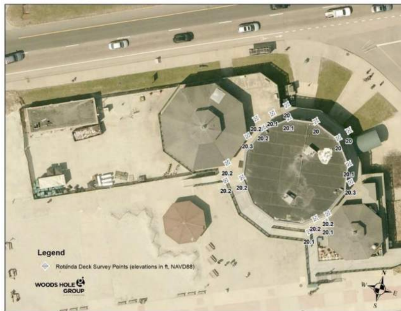
Figure 6: Critical elevations along the Deck surrounding the first habitable floor of the existing Rotunda.
